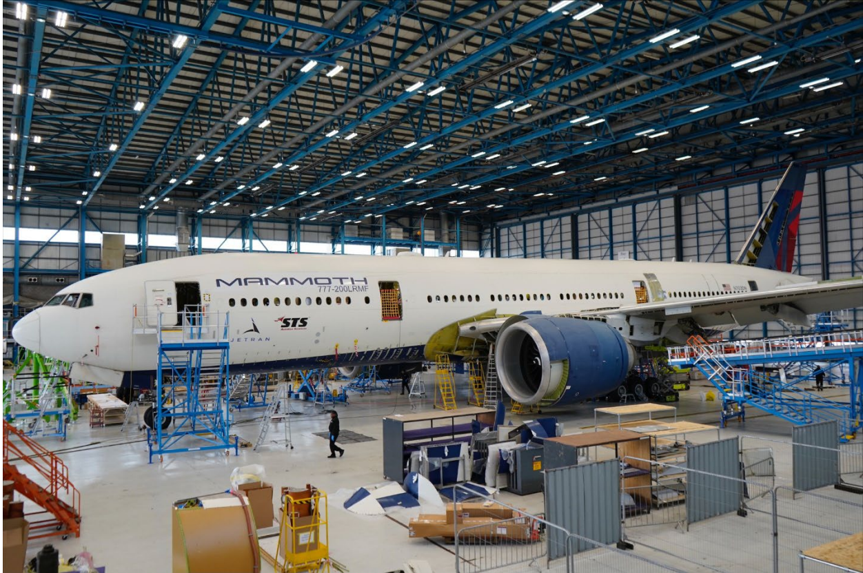
Mammoth 777-200LR (MSN 32222) undergoing conversion at STS Manchester.
